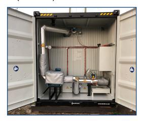
A FULLY SELF-CONTAINED MOBILE STORAGE SYSTEM FOR BITUMEN AND EMULSIONS
